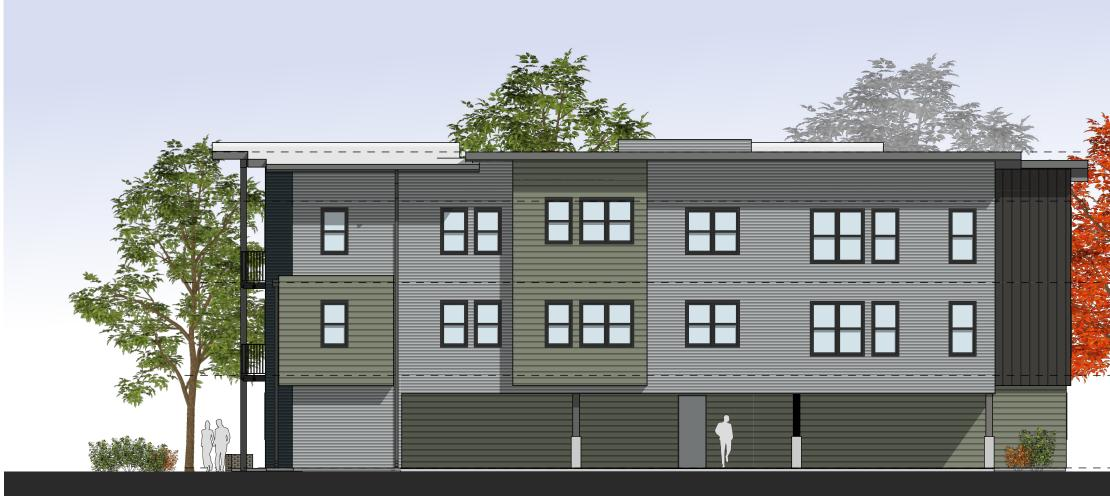
BUILDING A WEST ELEVATION BLDG. A1, A3, A5, A7 EAST ELEVATION - BLDG. A2, A4, A6 - SCALE 3/32" = 1'-0"
