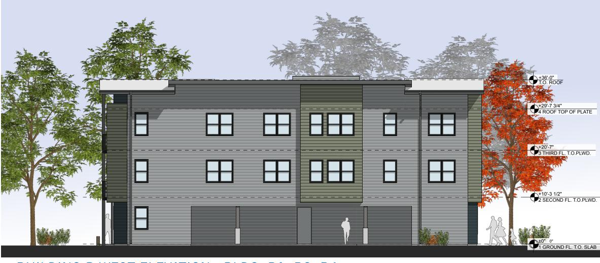
BUILDING B WEST ELEVATION - BLDG. B1, B3, B4 EAST ELEVATION - BLDG. B2 - SCALE 3/32" = 1'-0"
